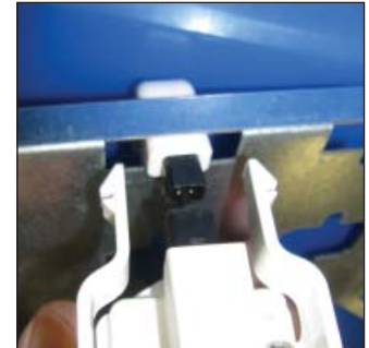
2. When the hooks are disengaged, pull the luminaire free.
